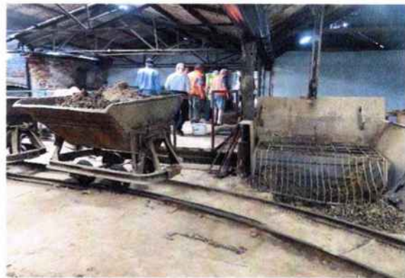
Fig.6 (left) Clay being delivered into a skip, running on a light rail system
