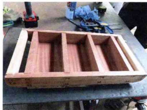
Fig.9 (right) A finished 3 mould box. Note the handles on either side for the hand maker to use when lifting and de-moulding.
