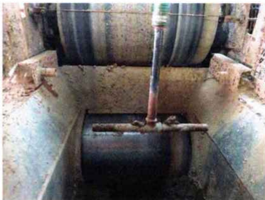
Fig.4 (left) Conveyor belt which will deliver clay to crushing and mixing rolls, with water added through the tee-bar nozzle.
