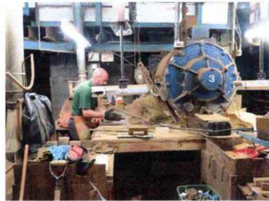
Fig.10 (left) A Berry Machine, used to carry out the final mix and tempering of the clay and delivering sufficient clay to the hand maker's bench.
