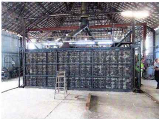
Fig.14 (left) The gas-fired intermittent kiln, holding 18000 bricks taking 3 days to fire a batch.
