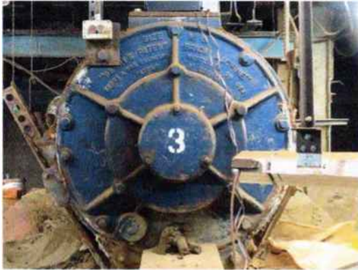
Fig.10 (left) A Berry Machine, used to carry out the final mix and tempering of the clay and delivering sufficient clay to the hand maker's bench.
