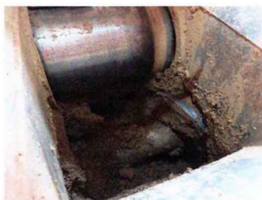
Fig.4 (left) Conveyor belt which will deliver clay to crushing and mixing rolls, with water added through the tee-bar nozzle.
