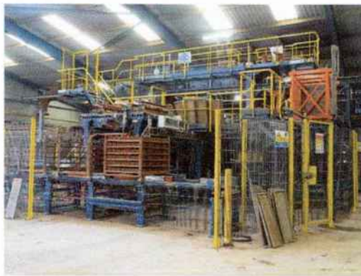
Fig.7 (left) Once the moulds are filled, they are assembled onto stillages in readiness for drying.
