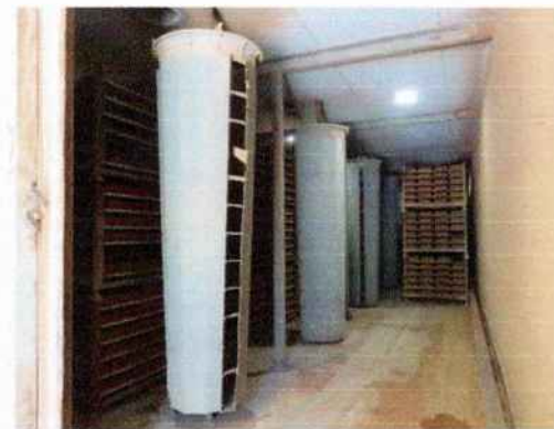
Fig.7 (left) Once the moulds are filled, they are assembled onto stillages in readiness for drying.
