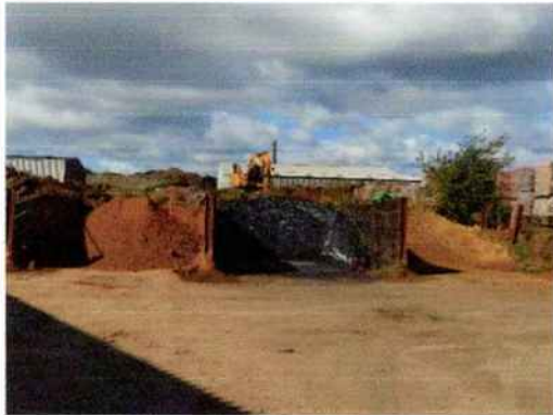
Fig.1 (left) Additive materials used in production. The centre bay holds coke breeze which is mixed into the clay body to aid kiln firing time and fired colour. The bays either side hold sands used for moulding.
