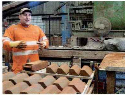
Fig.11 (left) Overview of the hand making line showing the large mixer, painted green, and the hand maker's bench.
