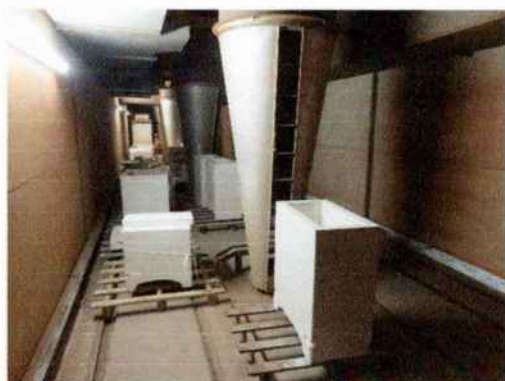
Fig.13 (left) Plaster of Paris mould sets being dried prior to use.
