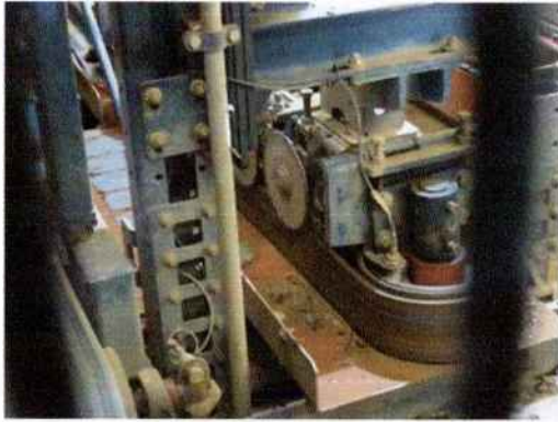
Fig.5 (left) Photograph looking down on the 'Striker Belt' which removes the excess clay from the mould boxes, with the material being re-cycled back into the mixer. The moulds are deliberately overfilled to ensure the actual mould box is filled with clay so that no air pockets exist.
