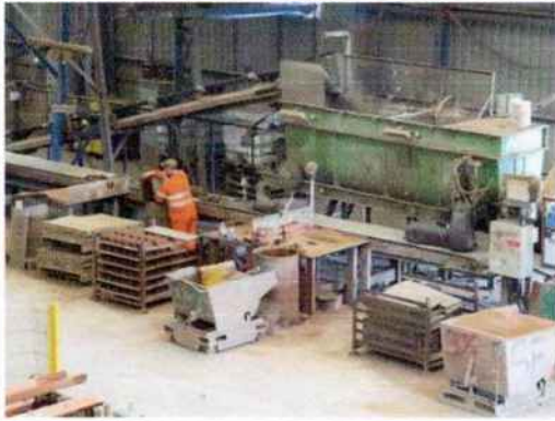
Fig.11 (left) Overview of the hand making line showing the large mixer, painted green, and the hand maker's bench.
