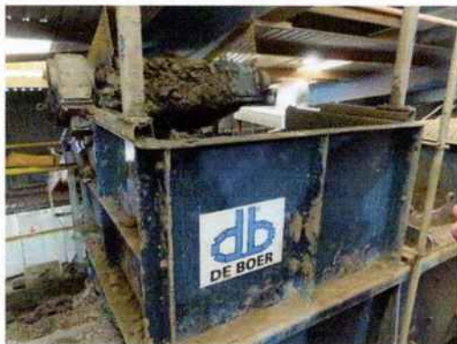
Fig.3 (left) The De Boer mixer where additional water is mixed with the prepared clay to ensure the correct moisture content is achieved. Typically, the Soft Mud Process requires around 21% moisture content. Any marked variation will result in either poor demoulding, if too dry or if too wet then slumping as the brick is de moulded.
