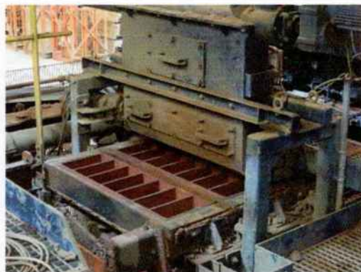
Fig.3 (left) The De Boer mixer where additional water is mixed with the prepared clay to ensure the correct moisture content is achieved. Typically, the Soft Mud Process requires around 21% moisture content. Any marked variation will result in either poor demoulding, if too dry or if too wet then slumping as the brick is de moulded.
