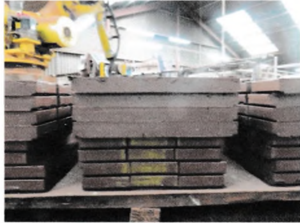
Fig.11 (left) Robotics used to commence the stacking of the cut tile.
