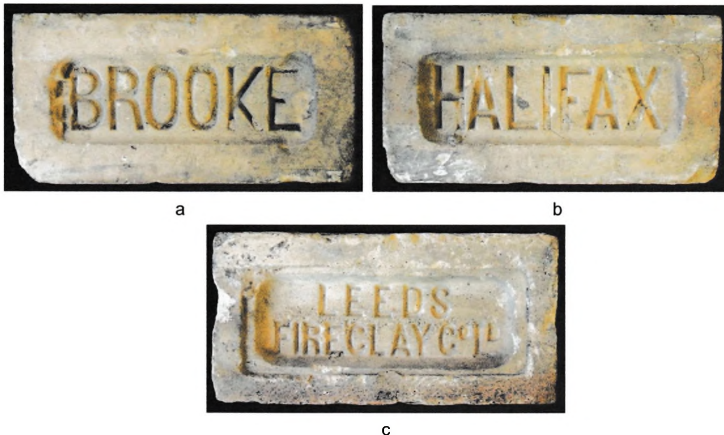
Fig.5 Sheffield industrial bricks: a and b, BROOKE/HALIFAX; c, LEEDS FIRECLAY C O L D
