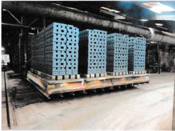
Fig.20 (left) Tiles set in “U” refractory cassettes, awaiting firing in the adjacent tunnel kiln.
