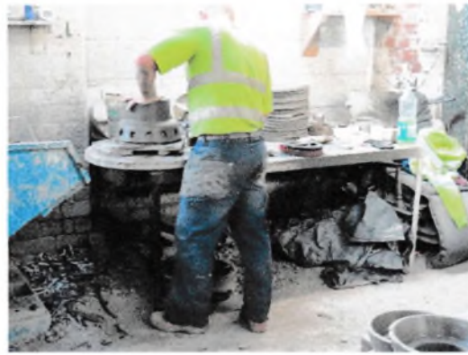
Fig.14 (right) Hand finishing, using a jig and boring tool to produce a flue vent, used to cap a redundant chimney flue.
