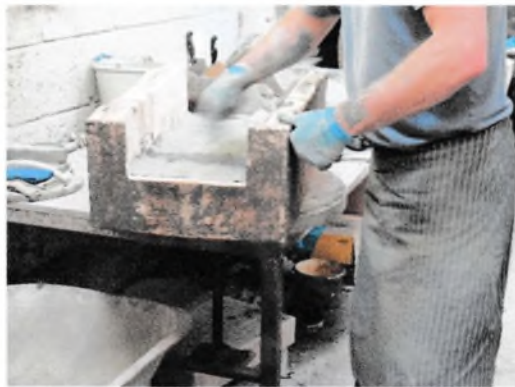
Fig.15 (left) Clay being carefully layered into one half of a mould
