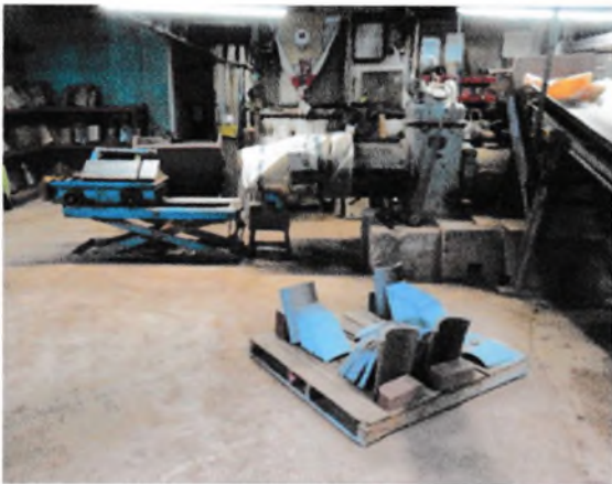
Fig.13 (left) Roof tile extruder being set up to produce ridge tiles.
