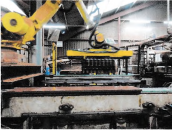
Fig.11 (left) Robotics used to commence the stacking of the cut tile.
