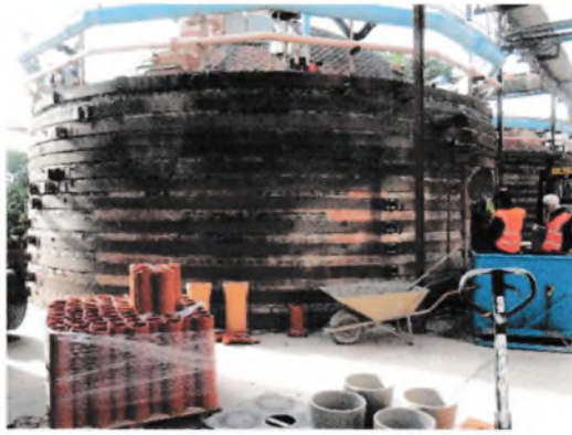
Fig.19 (left) Exterior of a Beehive kiln, showing the steel bands used to stabilise the structure during the expansion and contraction that occur during the firing cycle.
