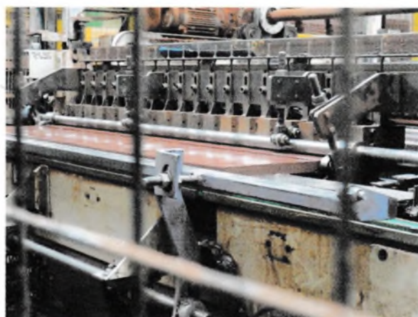
Fig.9 (left) Extrusion machine producing a continuous ribbon of tile.
