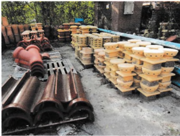
Fig.23 (left) The stock yard containing a wide variety of shapes and colours, including in the foreground gullies that have been salt glazed.
