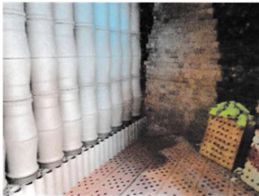
Fig.21 (left) A view of the kiln interior showing pots set on top of land drain pipes. The latter are used in most firings to help with stability. Despite severe competition from plastic, clay land drains are still in demand. The picture also shows the perforated refractory blocks, or 'Holey Boys' that make up the floor allowing the products of combustion to be removed from the kiln.
