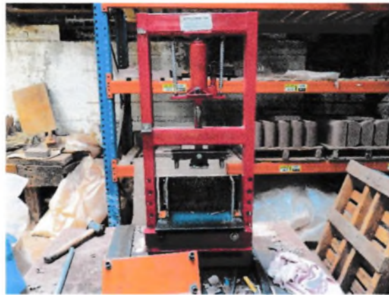
Fig.17 Hand-operated hydraulic press used for experimental shapes. The company is presently investing in an automated press line to manufacture new ranges of products.
