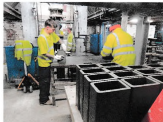
Fig.7 (left) Cavity liners in production being extruded on a hand-operated cutting table.
