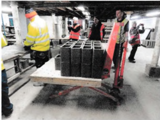
Fig.11 (left) Manual fettling station,with the orange coloured trolley being jacked to a level position so as to minimise operator lifting.
