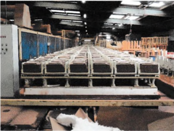
Fig.20 (left) Tiles set in “U” refractory cassettes, awaiting firing in the adjacent tunnel kiln.
