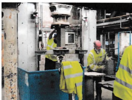
Fig.7 (left) Cavity liners in production being extruded on a hand-operated cutting table.
