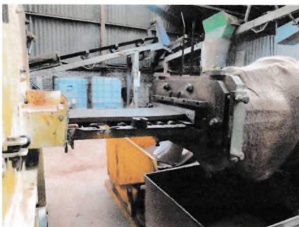
Fig.9 (left) Extrusion machine producing a continuous ribbon of tile.
