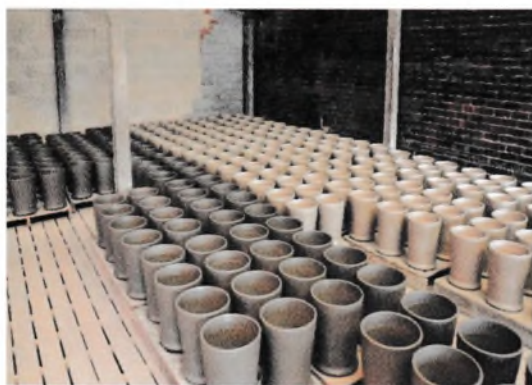
Fig.17 (left) A variety of pieces being dried, all placed on a slatted floor to facilitate the passage of warm air.
