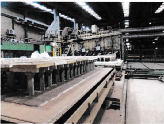
Fig.10 Left A general view of an unloaded kiln car,showing the unusual pedestal refractory deck design,which ensures that the development of the blue colour is even.In the background aone of the intermittent kilns has its hood raised from a hinge arrangement at the rear and giving it the appeance of the jaws of a crocodile.
