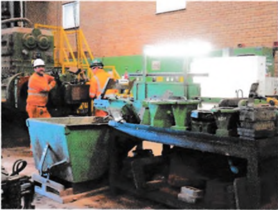
Fig.8 Left General view of the specials’ extruder, with the operators changing a die from the selection of shapes on the table.
