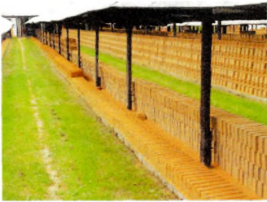
Fig.9 (left) An outdoor drying rack, with the bricks stacked to allow the circulation of air. Fig.10 (right) Alternative ways of stacking green bricks on the drying rack; skintled bricks are on the right giving maximum air flow.
