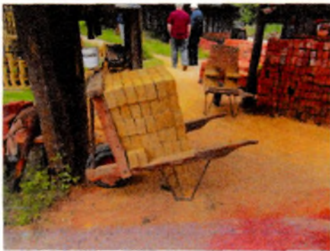
Fig.11 (left) A hack barrow loaded with dry, green bricks. Fig.12 (centre) The kiln set with the wicket entrance bricked up. Fig.13 (right) An internal bag wall.
