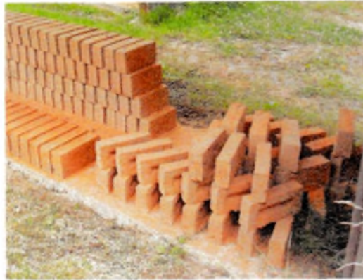
Fig.9 (left) An outdoor drying rack, with the bricks stacked to allow the circulation of air. Fig.10 (right) Alternative ways of stacking green bricks on the drying rack; skintled bricks are on the right giving maximum air flow.
