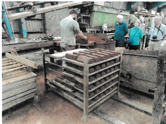
Fig.2 The handmade special shapes process being demonstrated.
