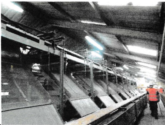
Fig. 10 Sieving the clay by means of wire screens.
