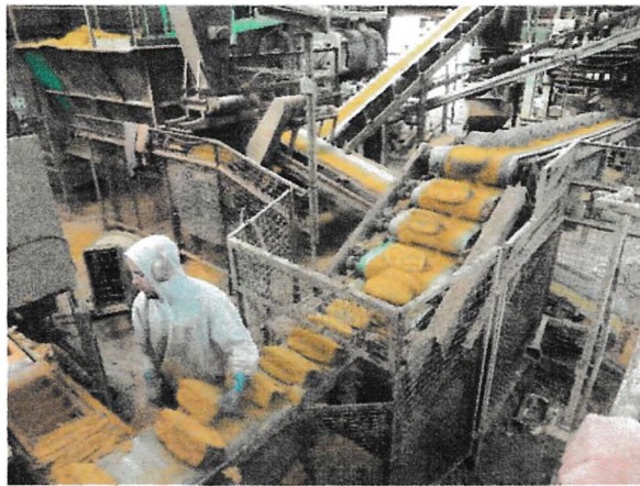
Fig.4 A hand maker with an empty mould set in front of him. As these hand makers have to work to the speed of the machine, they regularly rotate with colleagues to minimise fatigue.
