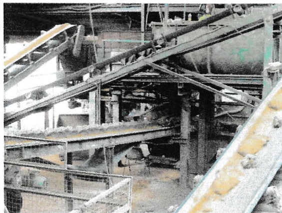
Fig.3 Prepared “walks” of clay ready for throwing on the mid photo conveyor, and in the foreground spare clay being conveyed back into the mixer for re use.
