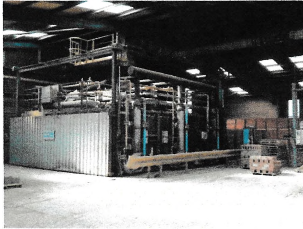
Fig.7 The Consultant Gas Equipment, CGE, kiln, firing temperatures for the local clay were 1000° C, whereas for the more refractory Williamson Cliff clay, this required a higher temperature of 1215° C.
