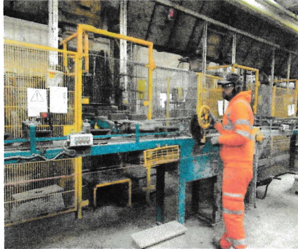
Fig.11 (left) Pressed bricks emerging from a Whittaker press, and automatically fed on to a conveyor system.
