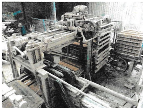
Fig.5 Wet bricks de-moulded and marshalled into packs ready for drying.
