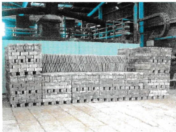
Fig.6 Packs of dry green brick, supporting floor tiles placed on the hearth of the Moving Hood kiln to form part of the next batch for firing.
