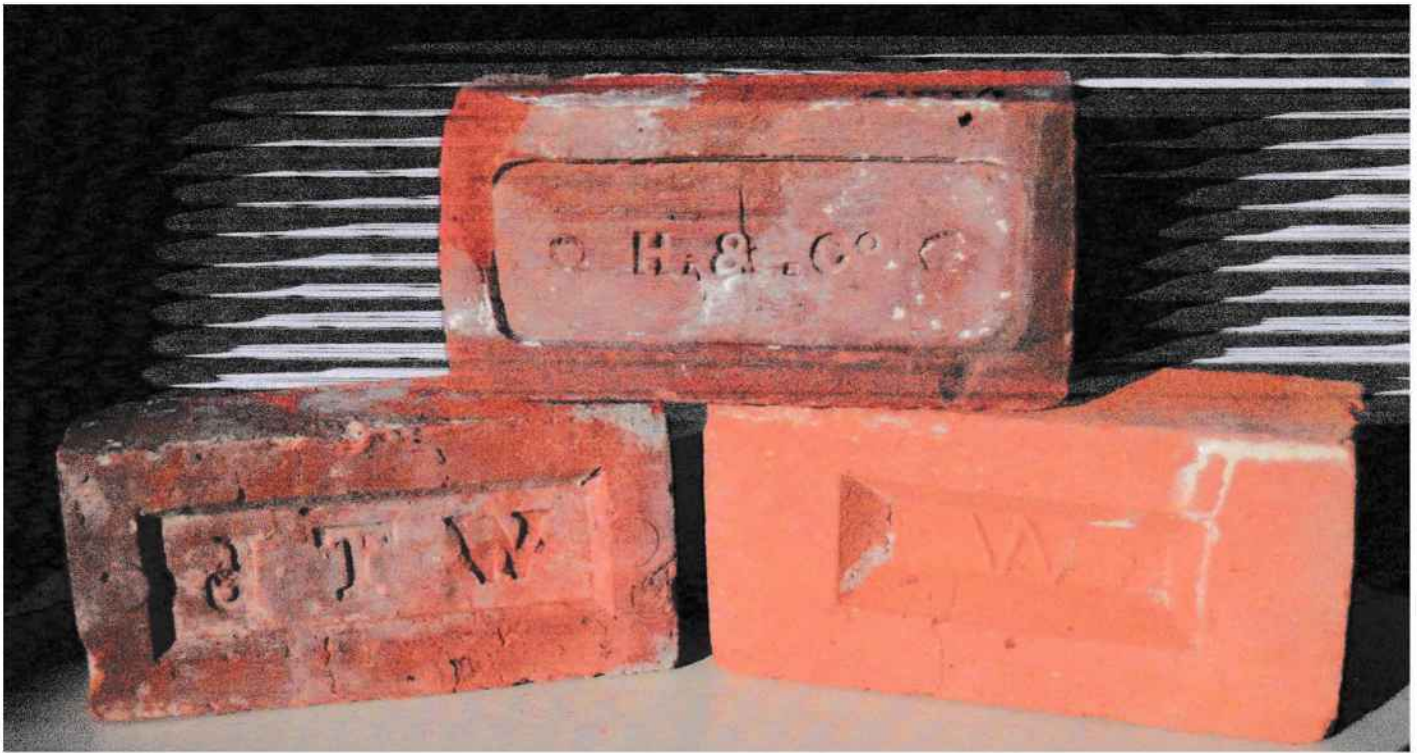
Fig.7 Bricks made at Chandlers Ford. That marked 'H & Co.' was made at the Hooper & Ashby brickworks.
