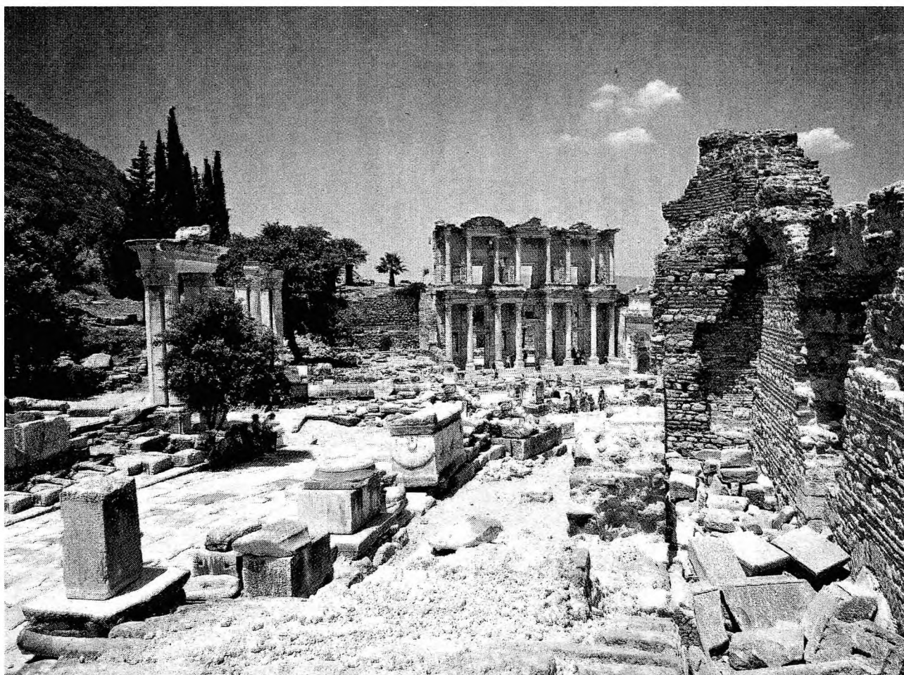
Fig. 1 Roman walling at Ephesus, Turkey, with brick and tile used as bonding material. This is on the right-hand edge of the photograph with the stage of the theatre in the background.
