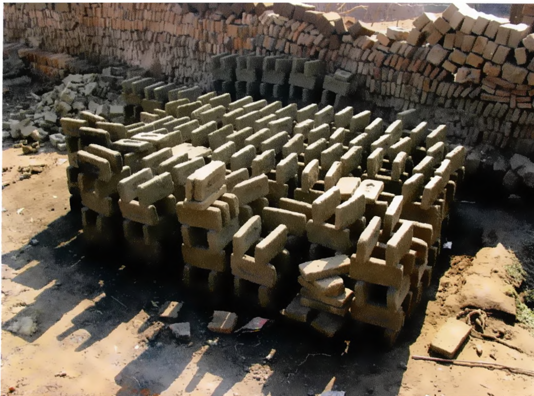
Fig.6 (upper) Initial drying: green bricks laid on the ground. Fig.7 (lower) Second stage of the drying process.
