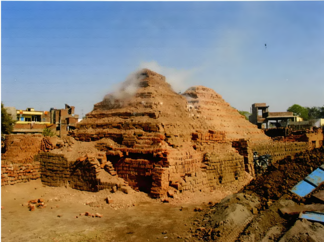
Fig.8 Firing in clamp kilns.
