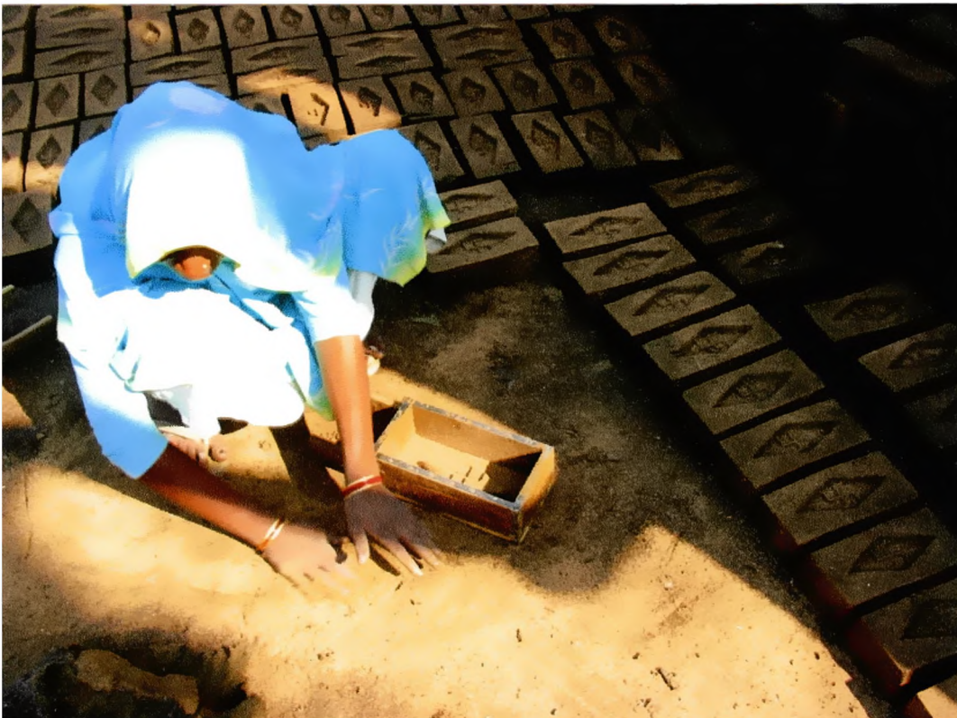
Fig.4 (upper) Timber brick moulds. Fig.5 (lower) The moulding process.
