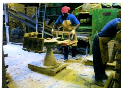
Fig.13 (left) 'Bearing-off' from the Berry machine table on to the dryer stillages.
