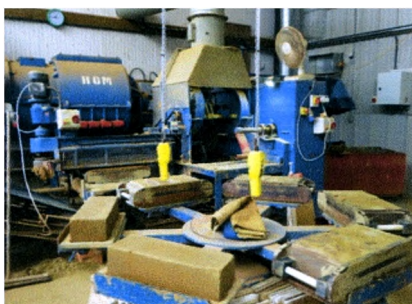
Fig.24 (left) 'Eco Blend' blocks, on table, marketed as 'Strocks Blocks', using a clay straw mix.
