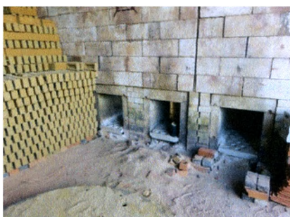
Fig.22 (left) Green set bricks, with the feed holes and refractory gates. Note the wood ash on the floor.
