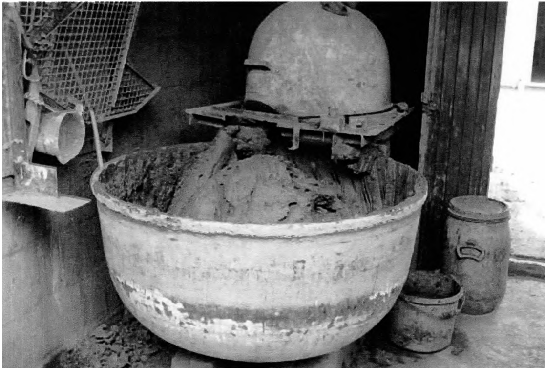
Fig.3 (above) The crushing and grinding layout. Fig.4 (below) Final mixing for hand throwing floor tiles (see also the cover).
