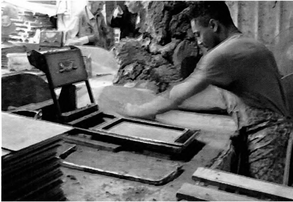
Fig.5 Tile production with hand throwing and pressing each tile into the mould. The raised lever to the left of the mould allows the Aldershaw trademark to be imprinted into the tile.
