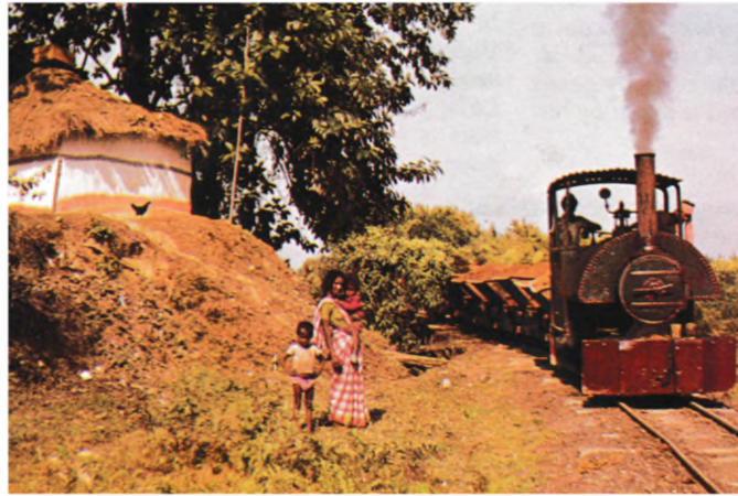
Fig. 3 A saddle tank engine pulls four tipper trucks either with raw clay or finished bricks along a narrow gauge railway on the Assam coalfield in the 1970s.
