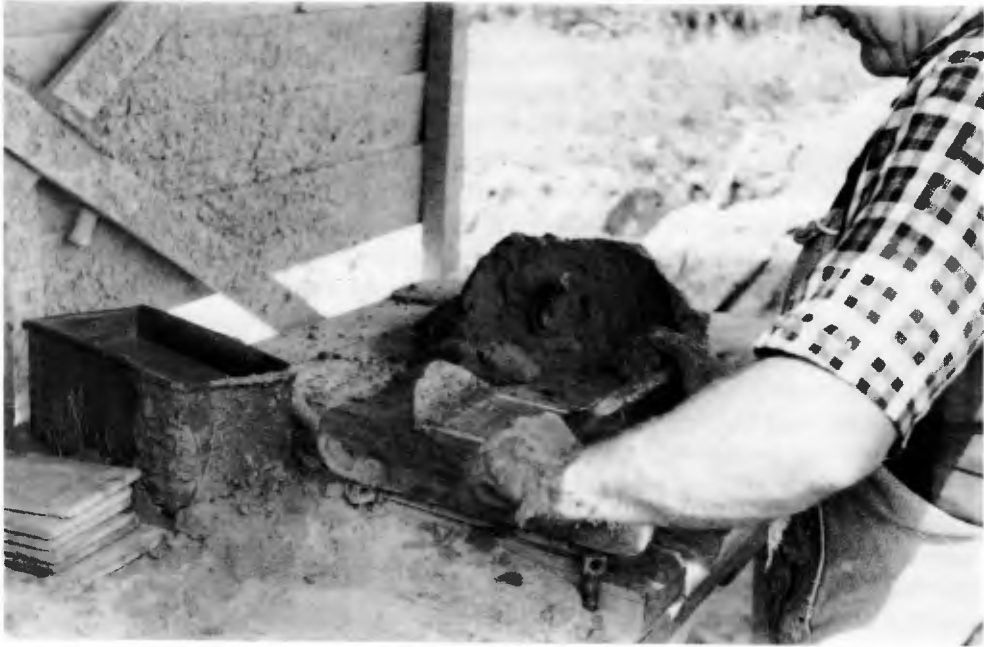
PLATE I Brick moulding using the strike
