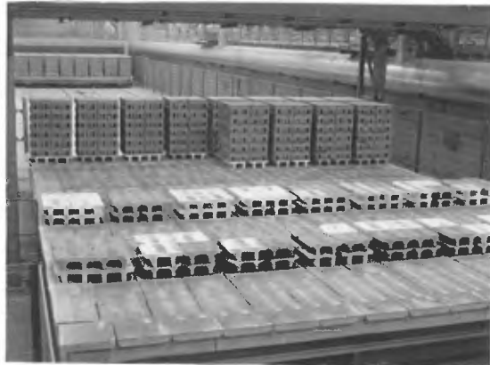
Fig. 7 (left) Robots building the packs of dry bricks; other robots placing the packs on the kiln cars.
