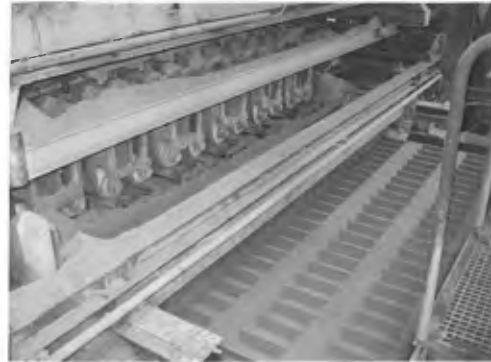
Fig. 5 (left) The 22 mould chain ready in a spare unit to minimise product changeover time.
