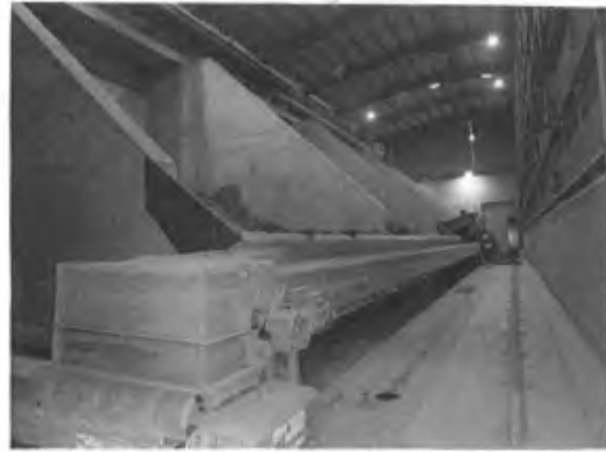
Fig. 3 (left) View of the main crushing rollers. This view of the equipment, open as it was undergoing maintenance, shows two of the quadruple roller arrangement, which is unique in the UK.
