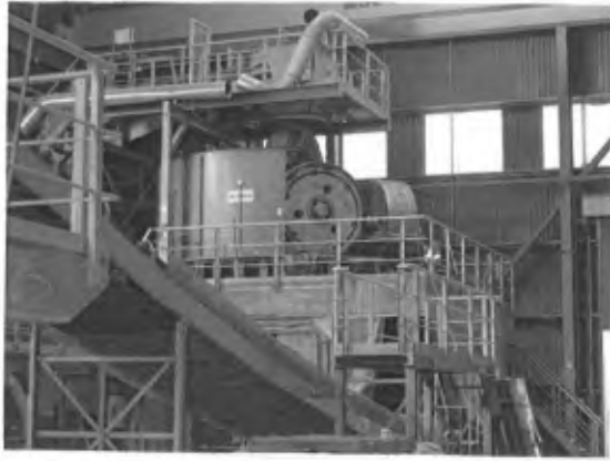
Fig. 3 (left) View of the main crushing rollers. This view of the equipment, open as it was undergoing maintenance, shows two of the quadruple roller arrangement, which is unique in the UK.
