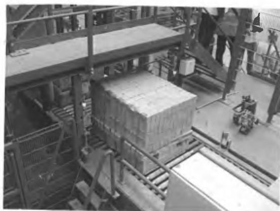
Fig. 8 (right) Packs of dry bricks placed accurately on the kiln furniture.
