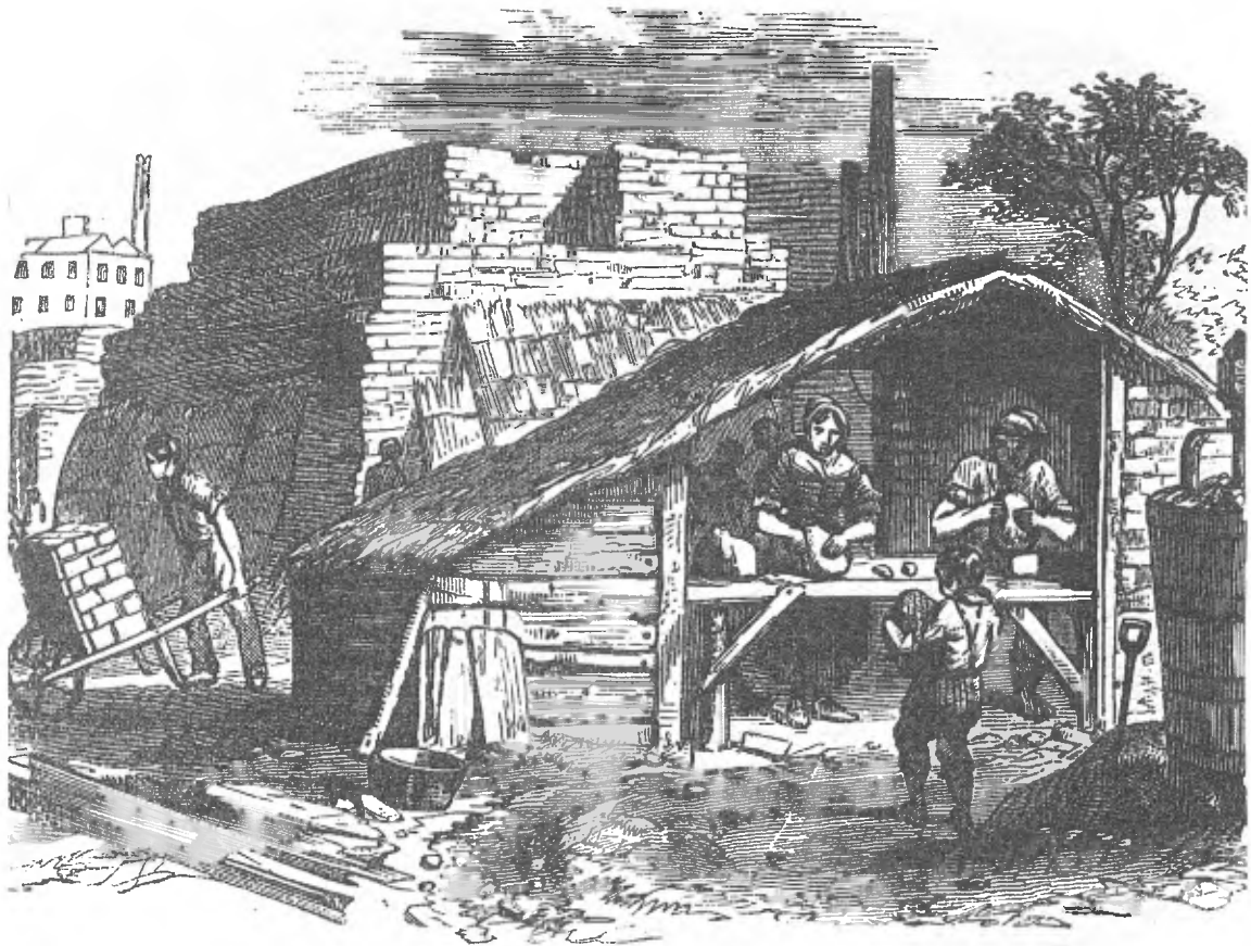
Fig.3. A nineteenth-century brickyard from The Boy's Book of Trades (1871). A man and woman (presumably husband and wife) are moulding bricks at a bench in a rough shelter of timber and thatch: a small boy (their son?) carries clay from the pugmill at far right, with the circular track walked by the horse also indicated; to the rear is a partly dismantled clamp and leaning against it are shelters which could be used on rainy days; at far left a man wheels away bricks on a barrow.
