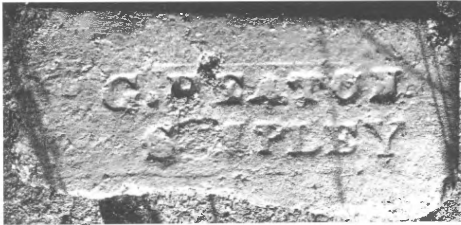
Fig.1 An example of an early frogless marked brick manufactured by George Heaton in the period 1856 to 1874. He is believed to have introduced firebrick making to Bradford.
