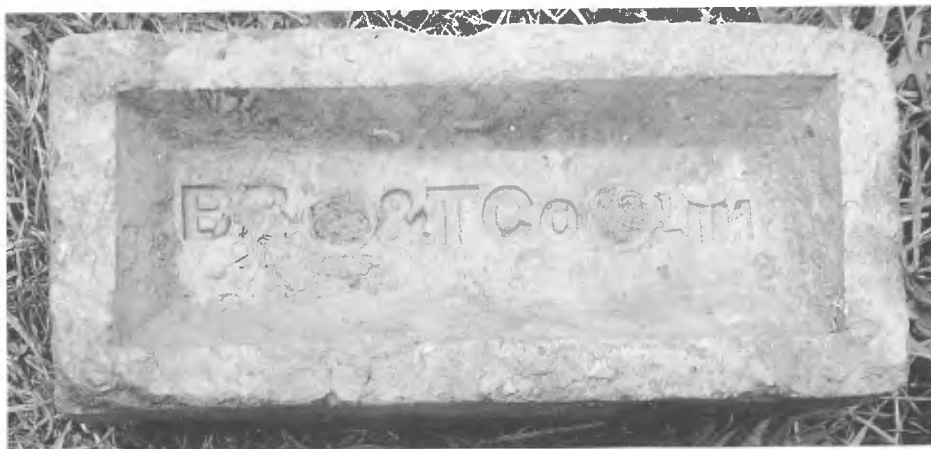
Fig.2 A later product of the Bradford Brick & Tile Company with the brickmark sitting in a frog.
