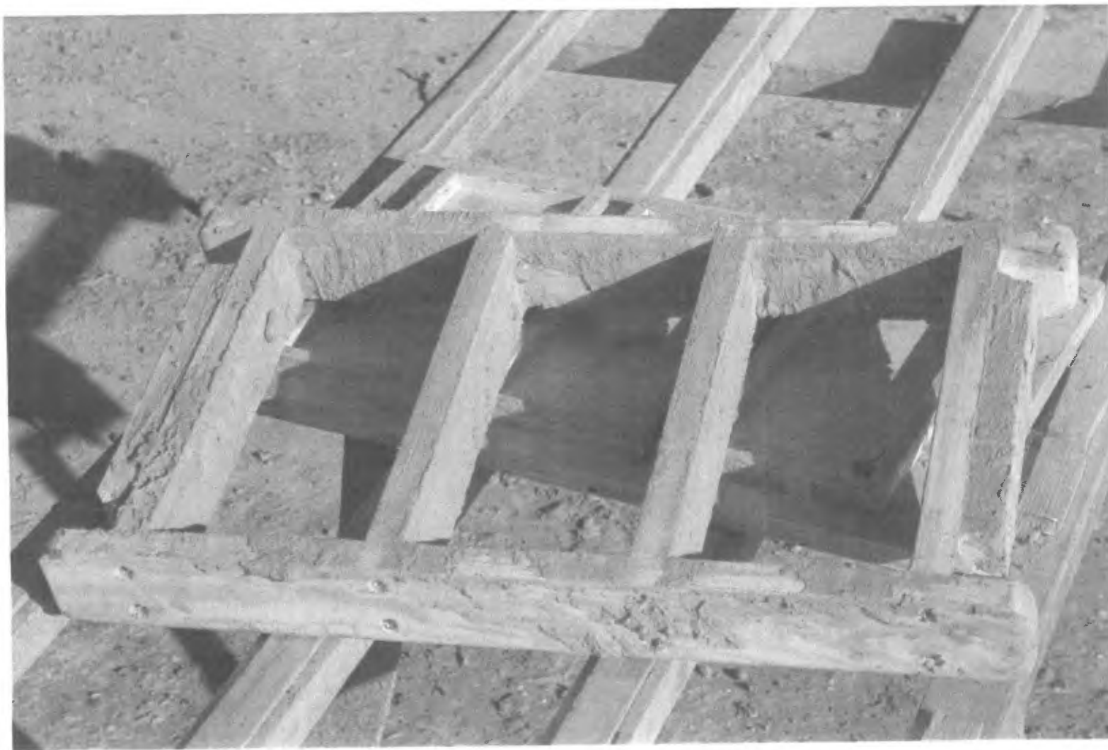
Fig. 3 New three-piece mould with the releasing board behind.
