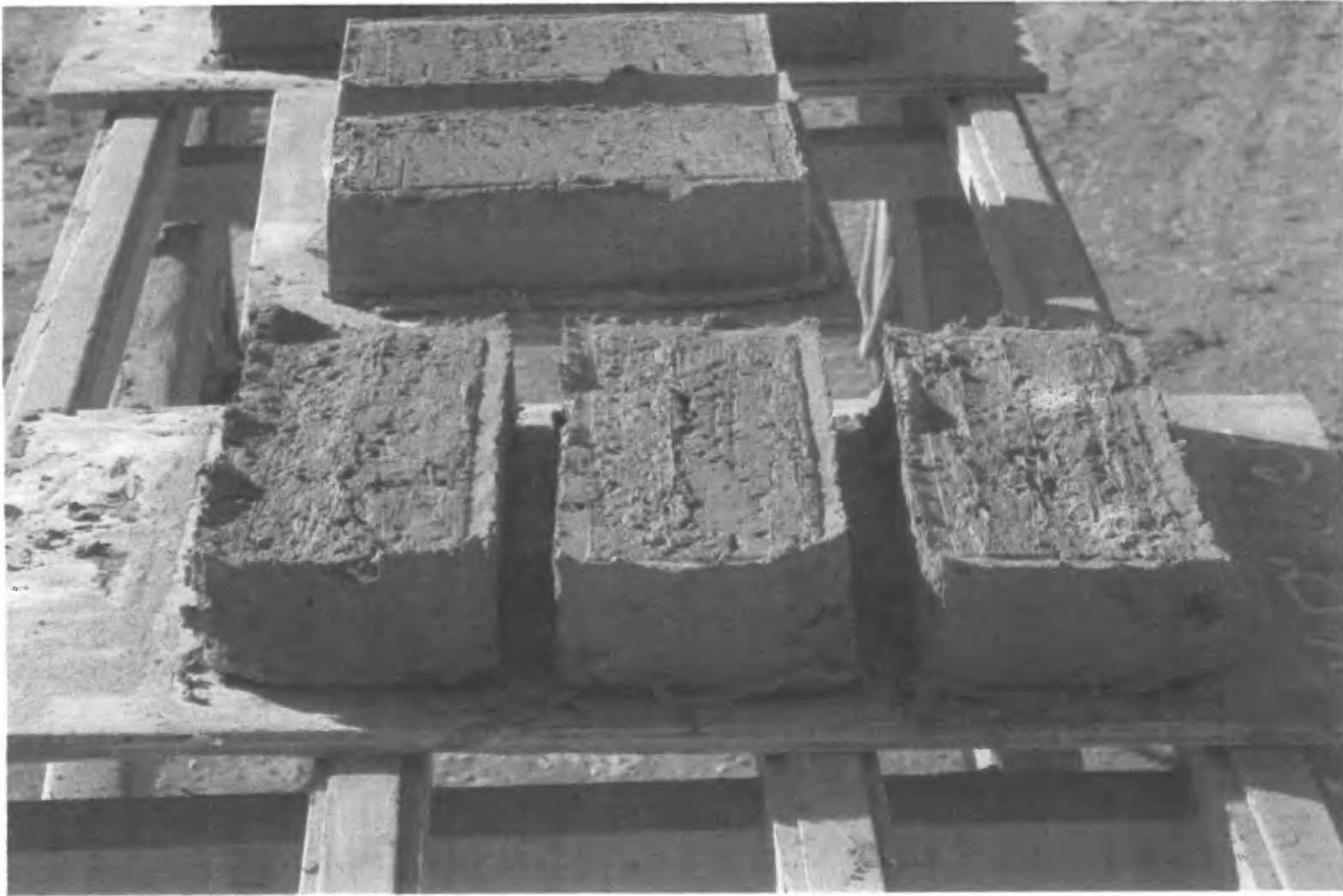
Fig. 1 Bricks made using slop-moulded unpugged clay, with the release board sanded, leaving sand on the margin.
