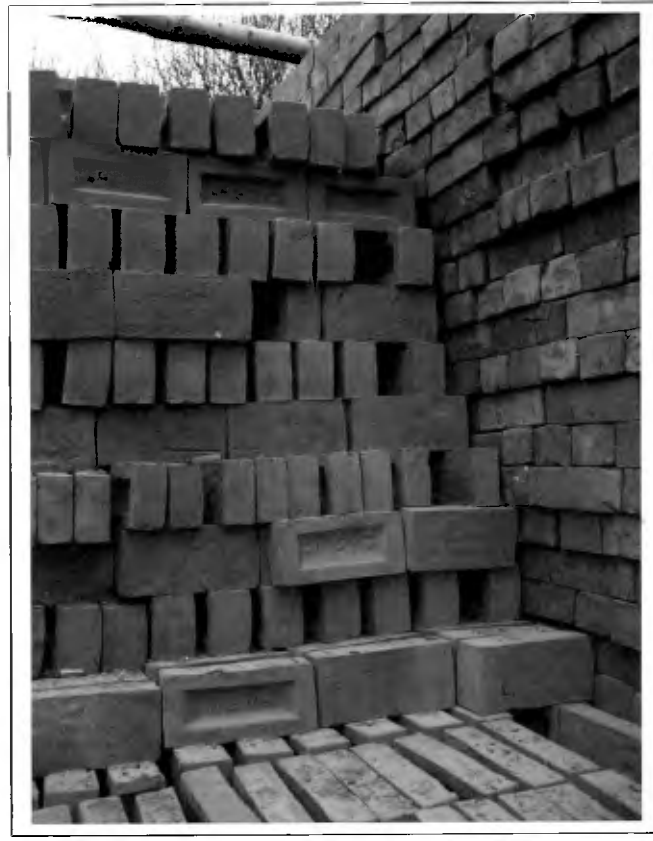
Fig. 1 The open-set bricks abutting the outer, un-mortared, wall or 'casing' of 'burnover' bricks.
