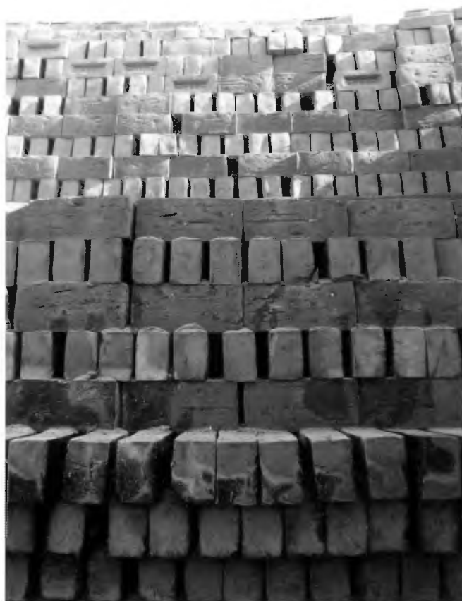
Fig. 8 The fired bricks from the wood-fired clamp-kiln displaying the potash-glazed bricks around one of the fire tunnels.
