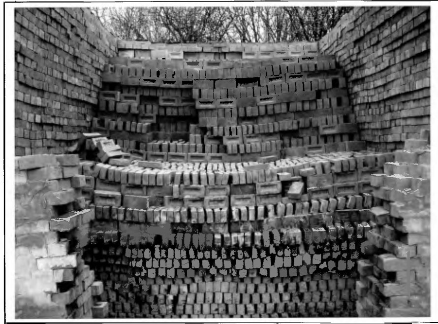
Fig. 5 A view through one end of the clamp after dismantling commenced where one can clearly see the potash-glazed headers that lined the fire tunnel at its base.
