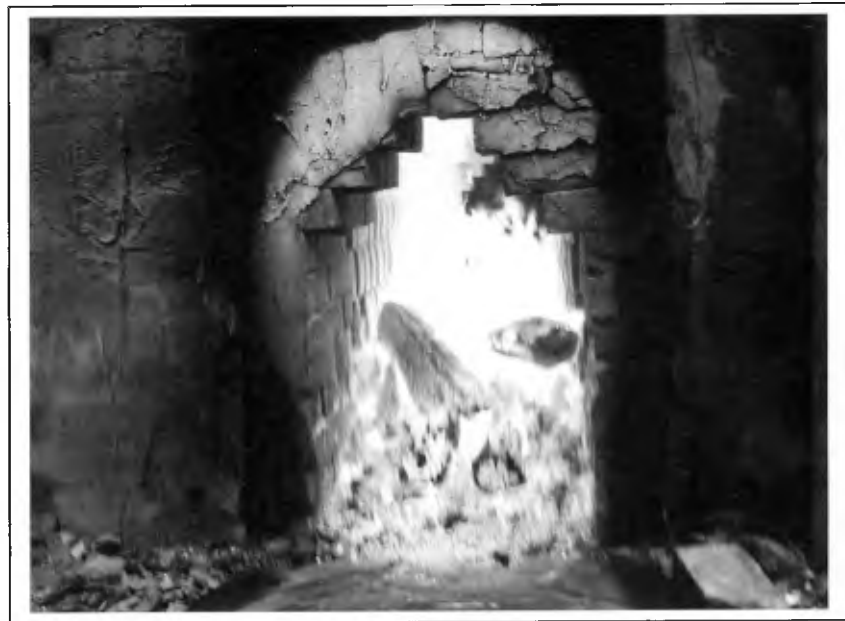
Fig. 4 The wood fuel placed at the mouth of the fire tunnel.
