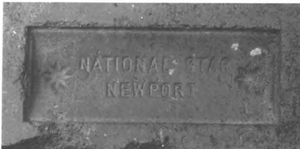
Fig. 2 Brick produced by the National Star Brick Company, Newport, with the company name and two stars in the frog.
